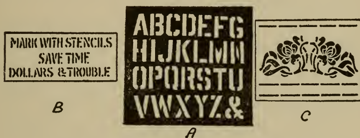
FIG. 82. STENCIL LETTERS AND STENCILS A. How stencil letters are cut. B. A stencil for marking boxes. C. Decorative stencil for wall borders.
